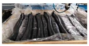
Thermoplastic, elastic, pressure sensitive sealant, for melt processing. Sealant DK-FR-P4E is designed for processing with a extruder. The material is self-extinguishing
