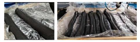
Thermoplastic, elastic, pressure sensitive sealant, for melt processing. Sealant DK-C1E / Sealant DK-T1E is designed for processing with a extruder. Extruder zones and extrusion heads should be equipped with temperature regulation. Recommended processing temperature should be in range of 80 - 120°C, temperature 160°C should not be exceeded due to possible material degradation.
